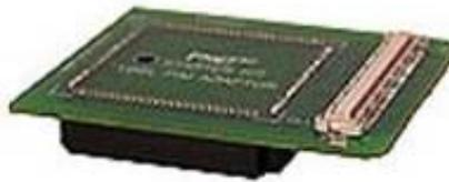
**Figura 5.23:** Adaptador “PIC32 Starter Kit 100L Pim Adaptor”.
