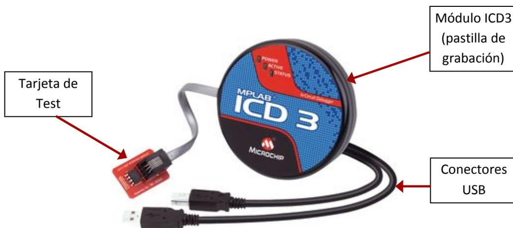
**Figura 3.14:** MPLAB ICD3 In-Circuit Debugger.
